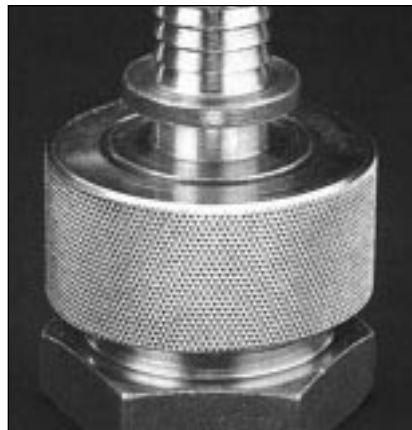
A round knurled Ground Joint Nut is available in ¾" and 1". It is useful for applications where less bulk and a low profile is desirable. Since the coupling is tightened by hand, the nut does not need bulky "handles" on the wing nut.
